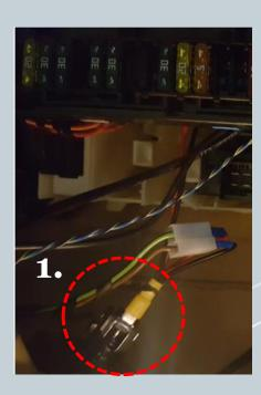
1. The supply for the WIC control unit can be taken from the 12V charging socket.
