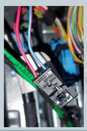
Insert the spun CAN cable into the plug provided. Thereby "blue / red" on pin\_1 and "red" on pin\_3. The numbering is marked on the plug.
