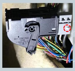
Use a small flat-head screwdriver to press and pull on the side of the pins. First press on the red marked area and pull out, then on the green area. Perform this procedure for each wire individually.
