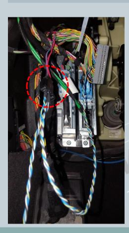
Connect the plugs (marked in red). The connector housing can be reinstalled and finally plugged back into the control unit.
