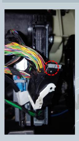
Unplug the black connector and pull it out of the connector housing. The housing is locked in from both sides (marked in red).
