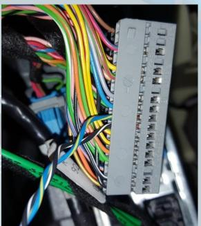
Pin the supplied CAN cable according to the picture.
