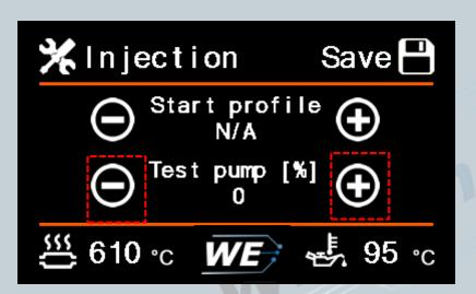
In this menu it is possible to check the functionality of the system and to make sure that the connection of the pump and the valves (if installed) was correct.
