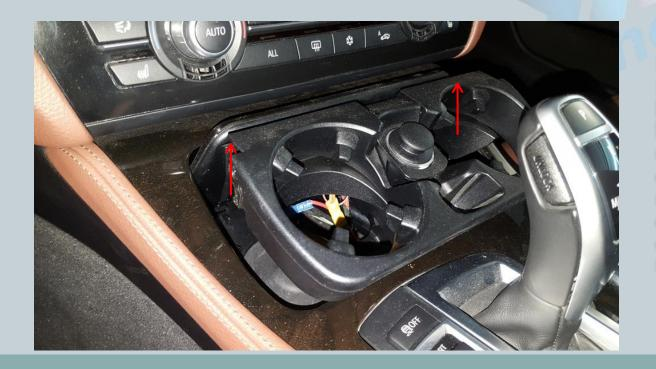
In the case of before the LCI model, the cup holder can be removed by simply pulling upwards. At the LCI the center console has to be removed to get the cigarette lighter. The center console is fastened with a screw.
