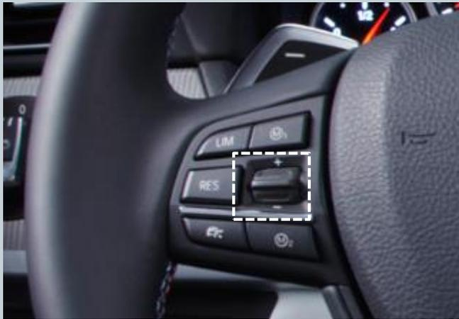
1. Use the paddles on the MFL can switch quickly between the individual screens. For this purpose, press the rocker slightly up or down.
