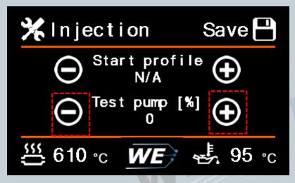
In this menu it is possible to check the functionality of the system and to make sure that the connection of the pump and the valves (if installed) was correct. Please disconnect the pressure line from the injection nozzle first and place the pressure hose in a small container. After activating the test function, liquid should come out of the pressure line.
