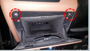
Loosen 2 screws on the storage compartment and pull out the compartment. The WIC control unit is located in this area.
