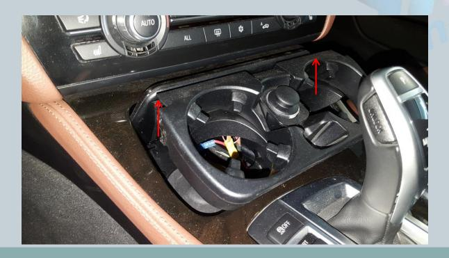
In the case of before the LCI model, the cup holder can be removed by simply pulling upwards. At the LCI the center console has to be removed to get the cigarette lighter. The center console is fastened with a screw.
