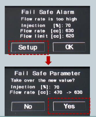
The display will show accordingly, at how many% injection control the error was detected. It also indicates which flow value was measured and the currently set flow limit.
