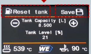
After each refueling, the tank must be reset with "Reset tank". Accordingly, 100% is displayed after tank tank level reset.
