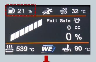
The tank contents must be specified to the system so that the rest of the tank contents can be displayed exactly. The WIC takes into account the amount withdrawn and calculates the remaining contents.
